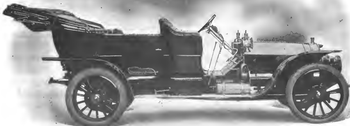
STODDARD-DAYTON MODEL G TOURING CAR, 6 CYLINDERS, 50-H.P., PRICE $4,500. Dayton Motor Car Co., Dayton, O.
